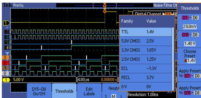
With the color-coded digital waveform display, groups are created by simply placing digital channels together on the screen, allowing the digital channels to be moved as a group. You can set threshold values for each pod of eight channels, enabling support for up to two different logic families.
