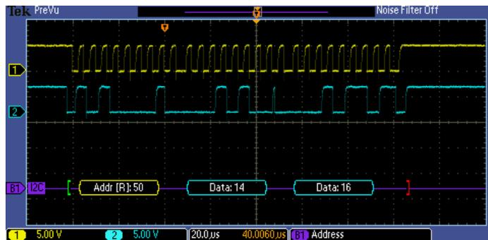
Triggering on a specific data packet going across an I<sup>2</sup>C bus. The yellow waveform is the clock and the blue waveform is data. A bus waveform provides decoded packet content including Start, Address, Read/Write, Data, and Stop.
