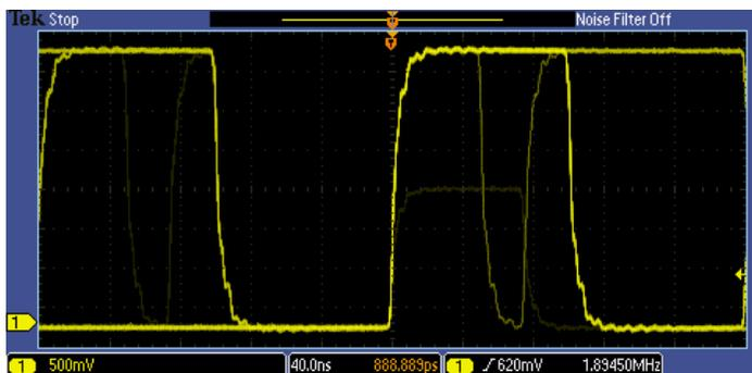
*Discover - A waveform capture rate of 5,000 wfms/s maximizes the probability of capturing exclusive glitches and other infrequent events.*
